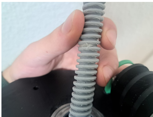
Figure 10.2: Image showing the Failure caused by the Full Load Test
