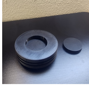
Figure 3.5: Image Showing the 3-D printed Piston head and Lead Screw Head
